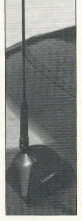
fact that the KG 2/70 was mounted at the very top of my rear window, while my other antenna was attached with a trunk lip mount, placing a major portion of the antenna element below the roof line.
